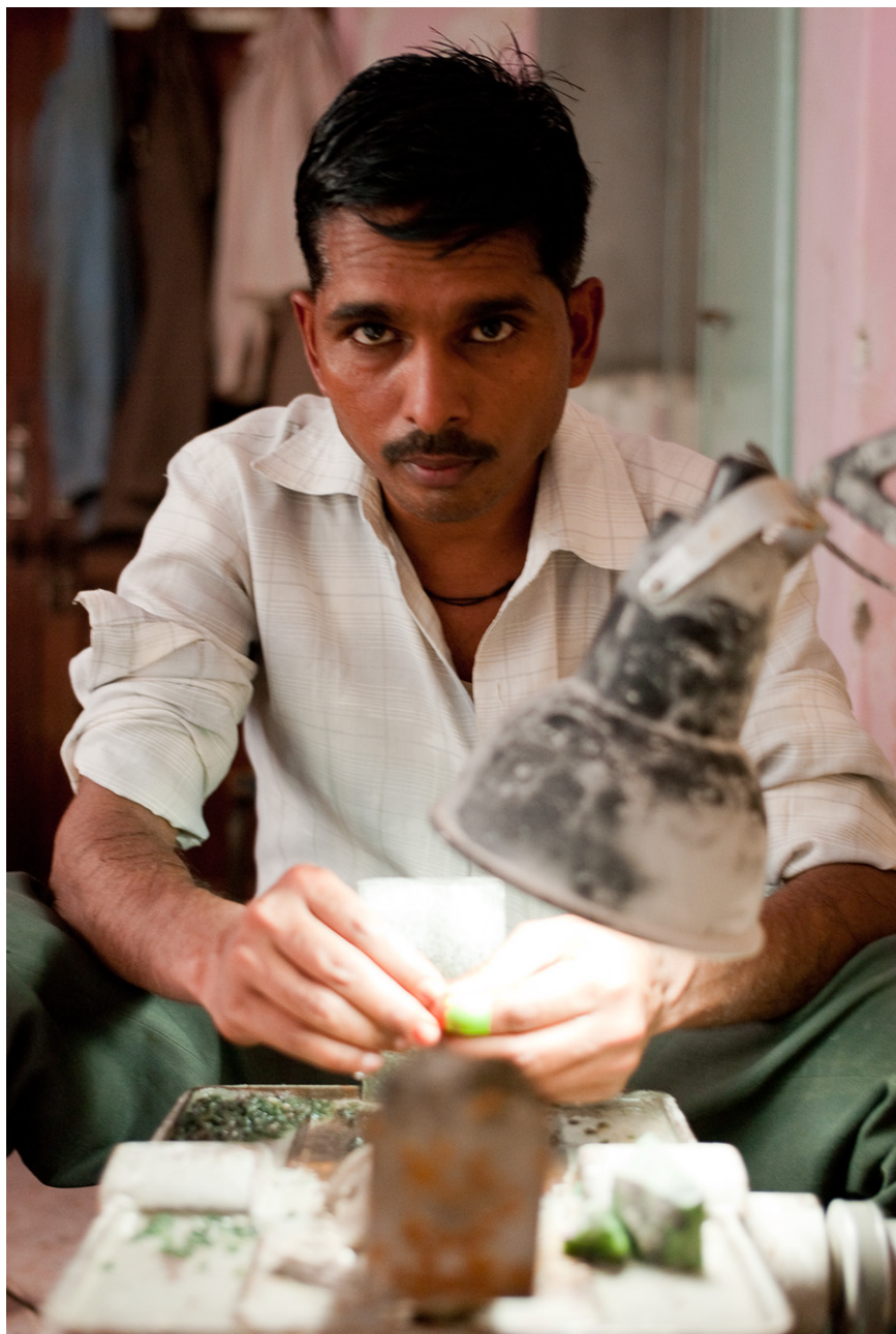
FIGURE 9. Karigar II. The stones are cut and polished in several steps. First, they are sawed on a spinning blade to separate the workable material from the uncolored beryl and the schist matrix.
